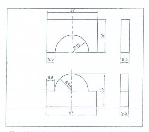
(Note: All dimensions are in mm and general tolerance is +/- 0.02mm.)
